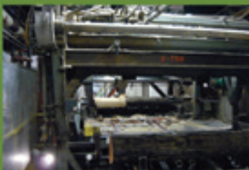
Before being peeled, the logs are debarked.
