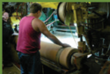
A high tech lathe peels veneer as thin as 1/42 inches from the logs.
