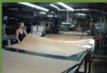
Veneer being graded and stacked by grade.
